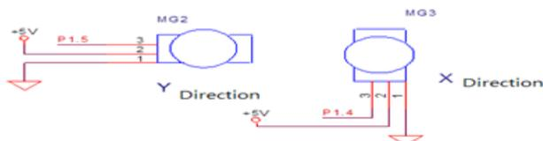
This servo motor signal wiring connect point, from the circuit we can see servo motor one wiring will connect 8051 (P1.4) and (P1.5) are X axis and Y axis respectively.
