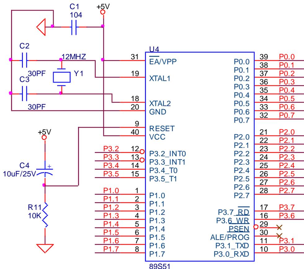
This is 8051, the port point connect a device to running overall system, they main for sunshine tracking to use and compare the sunlight value to change the solar panel turn angle. (Servo motor circuit)
