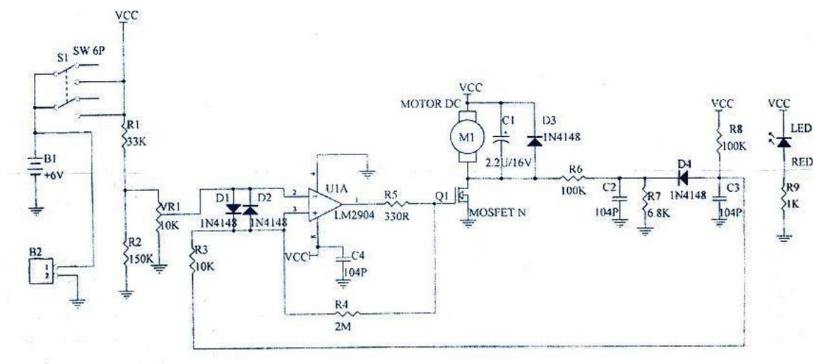
Through "pulse width modulation" (PWM) manner, by the output filter, and a comparator control, changing the size of the motor current received, and thus achieve the purpose of controlling the rotational speed
