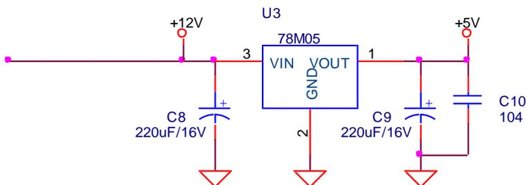
This is 5V power supply, The system is 12V change 5v to supply related device (LCD circuit connect to 8051 point)
