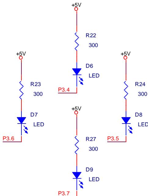
LED light a signal guide , when the tracking detect a direction to turn and the related LED light will on, we can know the panel turn which the direction
