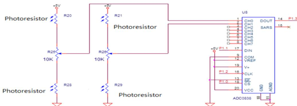
This is ADC circuit, use to analog change to digital value, by 4 photoresistor receives sunlight and compare the value send to 8051 (LED circuit diagram)
